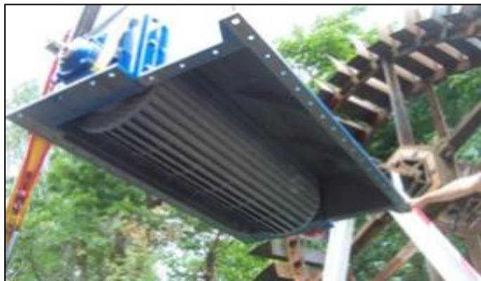
Figure 3.6: Cross-flow Turbine (HARET, 2018).
